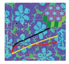
A thermodynamically stable phase separation of  $\text{Co}_2\text{Dy}_{0.5}\text{Mn}_{0.5}\text{Sn}$  into the Heusler compound  $\text{Co}_2\text{MnSn}$  and  $\text{Co}_8\text{Dy}_3\text{Sn}_4$  is induced by rapid cooling from the liquid phase. The phase separation forms an ordered flower-like structure on the microscale. The increased scattering of phonons at the phase boundaries reduces the thermal conductivity and thus improves thermoelectric and spincaloric properties.
