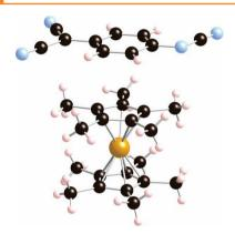
A new family of organic magnets with N,7, 7-tricyanoquinomethanimine (TCQMI) is reported. [Fe<sup>III</sup>(C<sub>5</sub>Me<sub>5</sub>)<sub>2</sub>]\*+[TCQMI]\*-forms parallel chains of alternating radical cations/anions and orders at 3.4 K as a weak ferromagnet. Amorphous M[TCQMI]<sub>2</sub>\*z CH<sub>2</sub>Cl<sub>2</sub> (M = V, Fe) have  $\mu_4$ -[TCQMI]\*-, and the Fe compound is a weak ferromagnet at  $\approx$ 4 K, whereas the V compound does not magnetically order.
