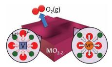
Formation of an oxygen vacancy (leading to a lattice contraction) with simultaneous cation radius increase (leading to a lattice expansion), which is investigated by atomic scale computational and empirical modeling, results in a chemical expansion of a non-stoichiometric oxide. Material compositions with minimal coefficient of chemical expansion, avoiding mechanical instabilities in high temperature applications, are predicted.
